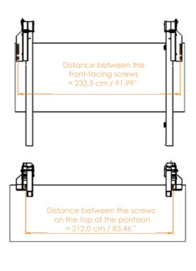
Remember that the minimum distance between the square tubes must be 191.7 cm/75.47 in and the minimum distance between the mounting plates must be 205.9 cm/81.06 in.
