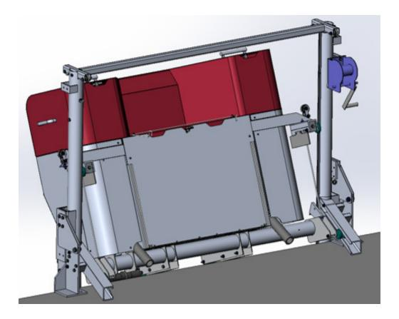
If the docking station option has been chosen, remove both panels as well as the round white tube assembly from the docking station before moving to step 4.
