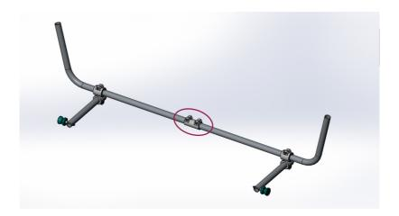
Align the tubes so that the curved tubes are in the same plane. Once everything is in position, tighten securely.
