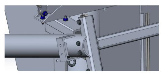
Assemble the reinforcing bracket (19) to link the upper right beam (5) to the pulley transfer beam (6).
