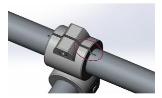
Repeat the process with the second **roller support (36)** and the second **half-cradle (37)** tube.
