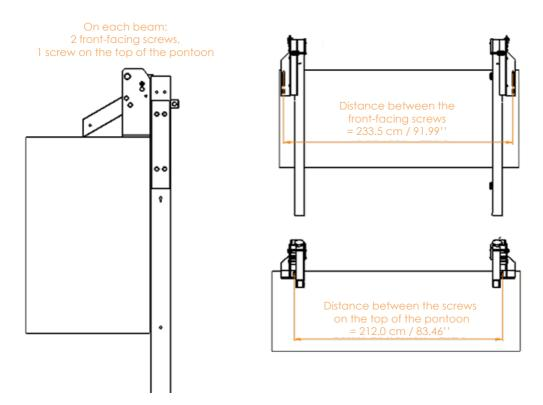
Remember that the minimum distance between the square tubes must be 191.7 cm/75.47 in and the minimum distance between the mounting plates must be 205.9 cm/81.06 in.
