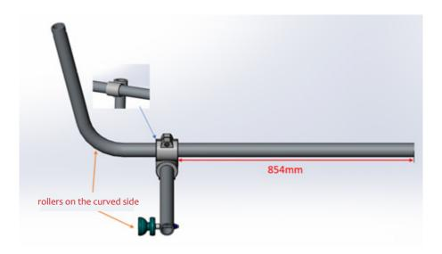
Make sure that the **roller support (35)** is perpendicular to the **half-cradle (37)** tube. The groove on the connector must be aligned with the line on the tube. Once it is positioned correctly, tighten the connector.
